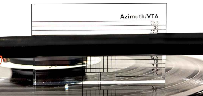
Pic. 1: Checking the VTA
